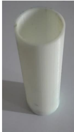
Figure 23 – Small 1.0 mm thickness test tube printed to validate glue less test.
